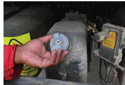
To reduce NOx level, 13 vehicles used on TARGET sites have installed AdBlue (Urea and water)
